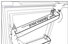
Press the right side of the door shelf inwardly, while holding the left side. When the notch of the shelf has been detached from the refrigerator door, remove the rack obliquely upwardly.
